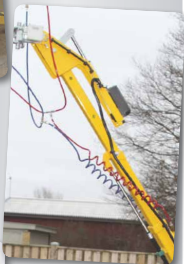
The beam has a manual extension in addition to the electrical.
