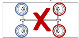
WARNING! If the suction cups are not connected diagonally, there is a risk of the load being pulled off the cups and the machine tipping over if one of the vacuum circuits fails!
